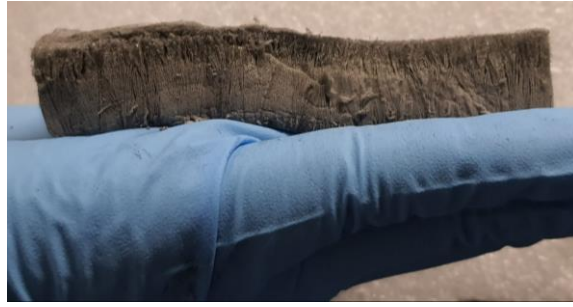
Figure 1 Digital image of aerogel sample fabricated using biomass materials by unidirectional freeze-casting.
